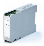
The MUH04-LF is a conductivity transmitter designed with an AC input amplifier and a galvanically isolated signal generator. The alignment of the conductivity electrode can be precisely adjusted by a potentiometer on the front. Temperature compensation of the measured value is available by a NTC-resistor within the measuring cell. The housing is suitable for rail mounting. The connection of the measuring cell as well as the power supply and the signal output are established by screw terminals.
